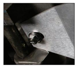
7. Now that the belly pan is attached at all three mounting points, go back and tighten the crash guard bolts and belly pan bolts. Re-install left side engine cover if you removed it.
