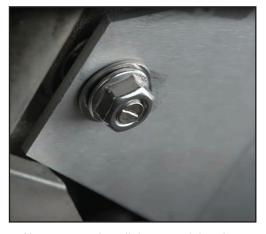
**4.** Now you can install the rear of the plate using the second M8 - 1.15 Serrated Flange Nut as shown
