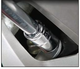
**5.** Remove front right engine guard screw, insert the right bracket as shown, tighten halfway. Attach the other end to the pan using the 5/16" Square Neck Carriage Bolts and Serrated Nylon Lock Nut. Slight twisting of bracket may be required on the right side.
