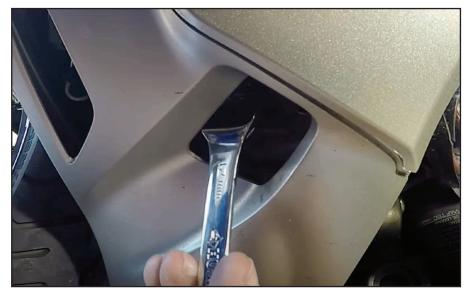
**6. OPTIONAL:** You can either remove the left side engine cover, or leave attached. If you do not remove it, the combination wrench is the best way to remove engine guard bolt. Repeat same steps as you did with the right side bracket
