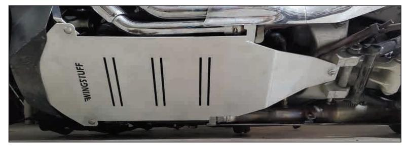
Tip: For oil change there is no need to remove the top engine guard bolts. Only the 3 screws that are attached to the bottom of the belly pan
