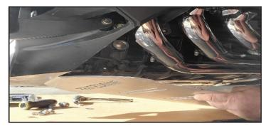
2. Push it inside the plastic cover about an inch. You can keep the belly pan on top of the plastic cover not tucked inside if you prefer
