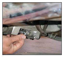
**4.** Insert the provided Rear T-Bolt through the existing oval hole in the center stand base of the motorcyle
