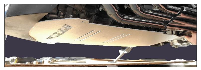
3. Slide the skid plate above the exhaust clips as shown in the picture above
