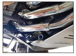
**10.** Adjust pan under the engine, tighten all screws and bolts. Re-install left plastic cover
