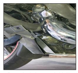
**9.** Remove the plastic cover on the left side. Front engine guard screw is not accessible like the right side. Repeat same steps for left side bracket as you did for the right side
