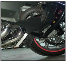
8. Remove front engine guard screw, insert the right bracket as shown, tighten halfway. Attach the other end to the the pan using the 5/16" Square Neck Carriage Bolts and Serrated Nylon Lock Nut. Repeat on the left
