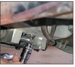
5. Use the thin flat nut with washer as shown, to go through the existing oval hole in the center stand base. Rotate T-Bolt inside the hole at a 90 degree angle and tighten the thin nut to hold the T-Bolt in place
