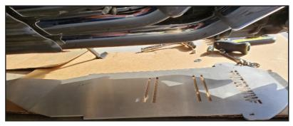
1. Slide the pan under the front plastic cover as shown
