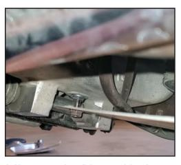
**6.** Now you can install the rear of the plate using the second M8 - 1.15 Serrated Flange Nut as shown
