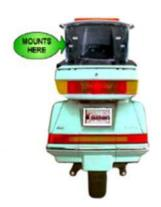
25LED can be plugged in-line with the connector on the back of the trunk lid as shown. Use Velcro strip to mount it.
