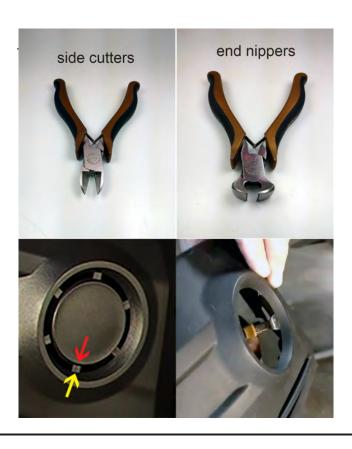
Note; the plastic on the cowl is a very soft material. If you apply pressure on it with a tool, it will turn white. Do not apply pressure to the material with your cutters until you are certain that you are in the correct position.
