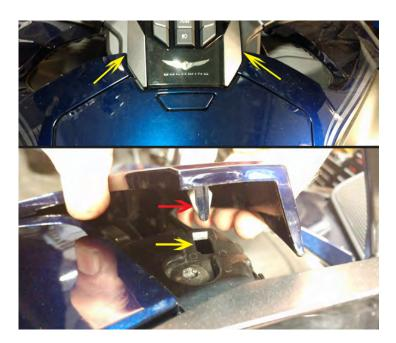
16. Use your 5mm allen wrench to remove the screw shown by the yellow arrow. You will have to remove the push pin shown by the red arrow. Pull on the center of the head until it pops up and then pull it out of its hole. (R)
