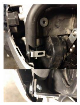
5. Assemble the left side light as shown. Note the brackets will be on top of the mount holes on the light. Also note the position of the wire. Tighten the screws slightly, but allow the bracket to slide.
