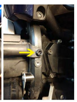
4. Attach the "L" bracket as shown using the supplied 10/32 x 1/2" screw and nylock nut. Note short end is against tab on bike. (R)
