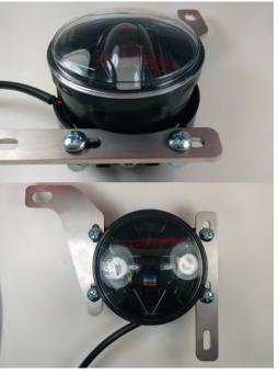
6. Assemble the right side light as shown. Note the brackets will be on top of the mount holes on the light. Also note the position of the wire. Tighten the screws slightly, but allow the bracket to slide.
