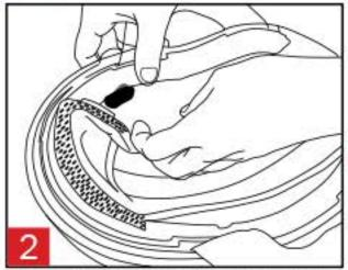
Peel and stick the female Velcro pads under your headliner inside the helmet on the left and right sides as diagram above.
