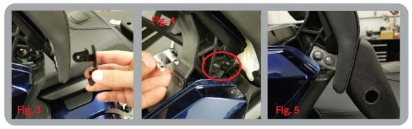
5. Slide the armrest into the hole where the plastic cover was removed and line up the holes with the attachment link. The hole in the rubber arm rest should face away from the bike. (Fig. 5) 6. Use two M6 x 20mm screws and washers to secure the arm rest.
