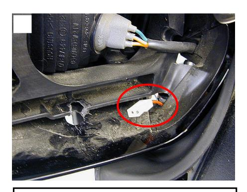
4. Insert supplied adapter harness into mirror housing by sliding the smaller connector through the hole as shown.
