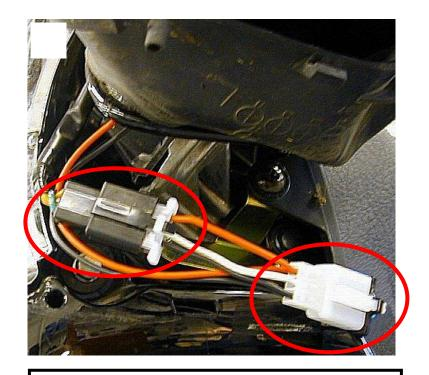
5. Connect the supplied adapter harness onto both ends of OE wires.
