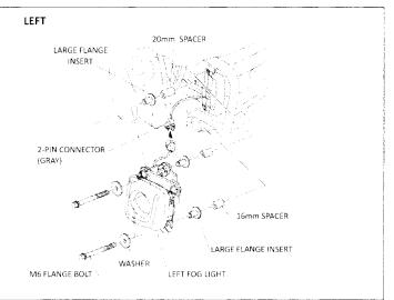
Note: There are six 2mm spacers in this kit. These extra spacers are for fine adjustment of your fog light as needed.
