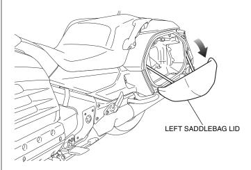
2. Remove the left side cover, and disconnect the negative (-) cable from the battery.
