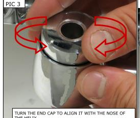
SECURELY HOLD THE HELIX, ROTATING ARM AND END CAP TOGETHER. MAKE A MARK ON THE END CAP AND ARM
