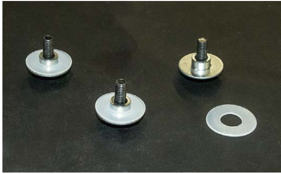
Windshield Flange Bolts and Nylon Washers Removed.
