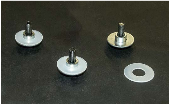
Windshield Flange Bolts and Nylon Washers Removed.
