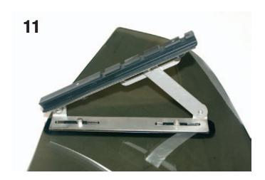
(fig 12) Before you put your Top Shield back on the bike, you may want to protect the windshield garnish with tape as the shield will be loose and could slide into the paint.
