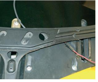
Plug the actuator into the extension harness.
