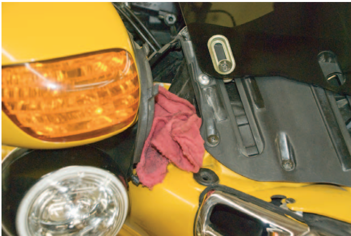
The VERY important rag location. Windshield Garnish and Clamp are removed in this photo.
