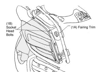
Install the left wind deflector (2A) by aligning the mounting brackets (2C) with the holes where the two fairing screws were removed. Two M5-0.8 x 16mm socket head bolts (1B) have been provided for installing each deflector. Use thread locking compound on the mounting screws. Do not over tighten.
