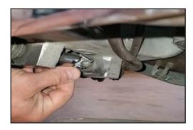
1. Insert the provided Rear T-Bolt through the existing oval hole in the center stand base of the motorcyle
