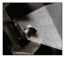
7. Now that the belly pan is attached at all three mounting points, go back and tighten the crash guard bolts and belly pan bolts. Re-install left side engine cover if you removed it
