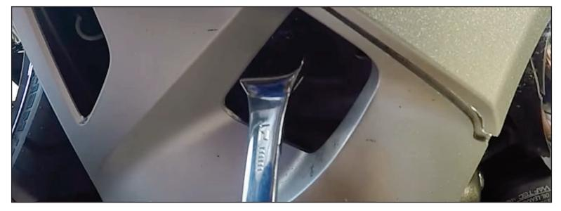
**6. OPTIONAL:** You can either remove the left side engine cover, or leave attached. If you do not remove it, the combination wrench is the best way to remove engine guard bolt. Repeat same steps as you did with the right side bracket
