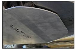
OPTIONAL: You can either keep the front of the belly pan tucked inside or outside of the front lower cowl
