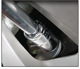
**5.** Remove front right engine guard screw, insert the right bracket as shown, tighten halfway. Attach the other end to the pan using the 5/16" Hex Drive Bolts and Lock Nut. **OPTIONAL:** Brackets can be attached using either end. Also, in or outside of mounting tab
