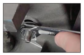
2. Rotate T-Bolt inside the hole at a 90 degree angle and tighten the thin flat nut to hold the T-Bolt in place
