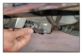
1. Insert the provided Rear T-Bolt through the existing oval hole in the center stand base of the motorcyle
