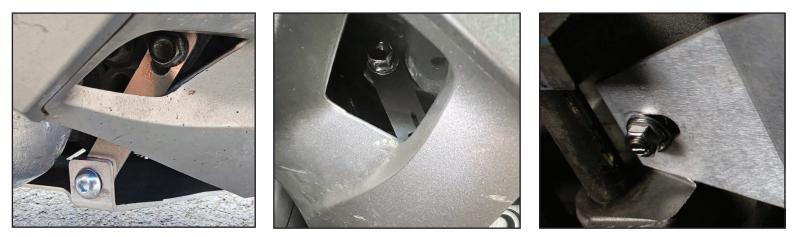
7. Now that the belly pan is attached at all three mounting points, go back and tighten the crash guard bolts and belly pan bolts. Re-install left side engine cover if you removed it
