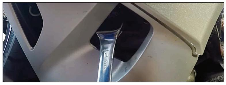
6. OPTIONAL: You can either remove the left side engine cover, or leave attached. If you do not remove it, the combination wrench is the best way to remove engine guard bolt. Repeat same steps as you did with the right side bracket
