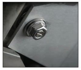
4. Now you can install the rear of the plate using the second M8 - 1.15 Serrated Flange Nut as shown and tighten halfway
