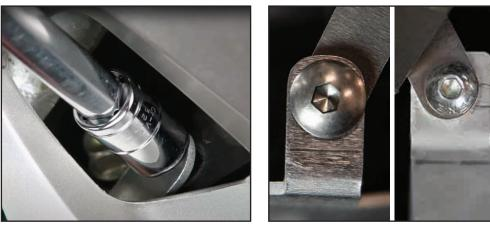
5. Remove front right engine guard screw, insert the right bracket as shown, tighten halfway. Attach the other end to the pan using the 5/16" Hex Drive Bolts and Lock Nut. OPTIONAL: Brackets can be attached using either end. Also, in or outside of mounting tab
