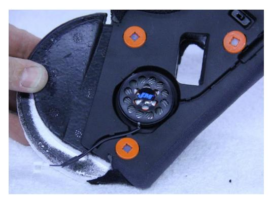
8. Reinstall both left and right-side styrene cheek-pads and while sliding them back into place, plug both speakers and the microphone into the main wiring harness of the headset. Use the supplied wooden tool to slide each wire under the main neck-roll and cheek pad interior padding, out of site.
