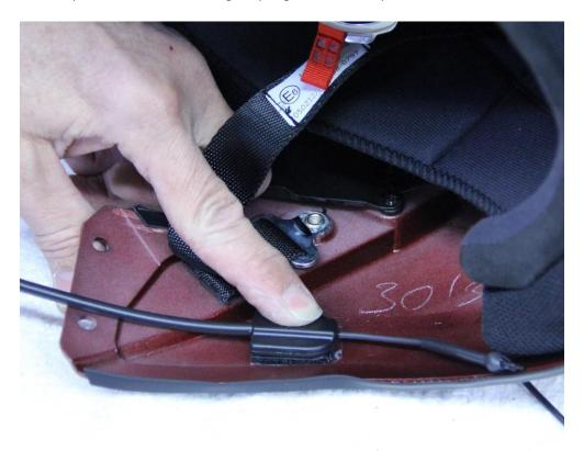
6. Peel the backing off the large Velcro pads and place them into the bottom of each speaker pocket indent for both left and right-side styrene pads as shown.
