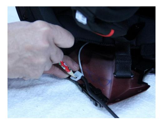
3. Drill the hole from the outside, using a small hand drill and it is recommended to drill the hole to 1/8" size first, before stepping up to the 5/32" drill bit.
