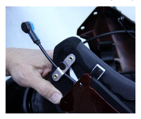
9. Now reinstall both left and right-side interior padding pieces and secure to complete the installation.
