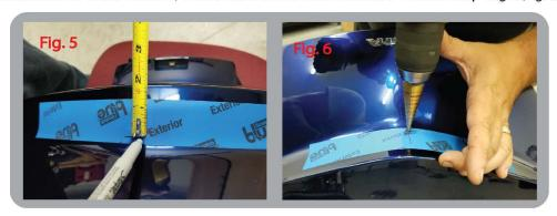
7. Drill a 9/16" hole where you marked the trunk lid, large enough to feed the connectors through. A step drill works well for this. (Fig. 6)
