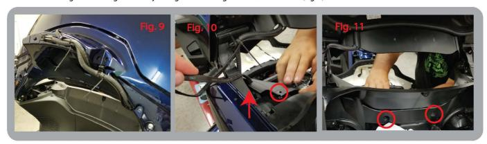
13. Open the saddlebags and remove the two side panels below the seat. Unplug the heated seat harness (Fig. A). Using a 6mm allen wrench, remove the seat screws on each side (Fig. B). Pull straight up on the front of the seat then slide the seat forward to release the rear of the seat.
