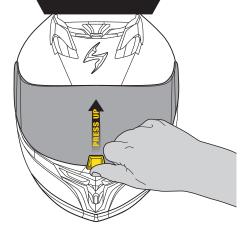
TO OPEN: Unlock the faceshield by pressing your thumb up on the faceshield lever until it snaps open. Lift faceshield all the way up.
