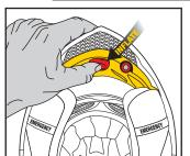
**DEFLATION:** Press the small pressure release button located beside the pump. **DO NOT** attempt to remove your helmet before deflating the air bladders.
