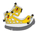
**M** NOTE Make sure snaps are in the down position before reinstalling
