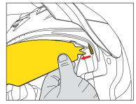
Firmly hold the SunVisor with your hand and gently pull one side out away from the helmet to release. Repeat to release the opposite side
