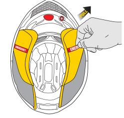
Locate the emergency labeling on the neck roll. Simply reach under the neck roll and grab the release strap, pull at a 45° degree angle towards the front of the helmet. The cheek pads will easily release from the helmet. This system should only be used by a trained medical personal.
