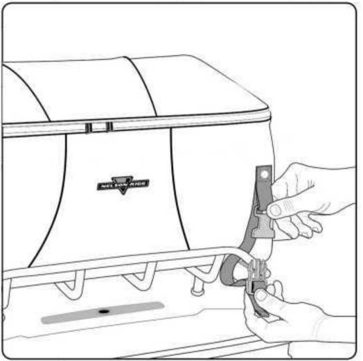
Position bag flat on your luggage rack making sure the bag is centered and free from any moving parts. Pass the strap with the male buckle around the luggage rack or post and reconnect back into the female buckle attached to the bag.Make sure the male buckle clicks into place when inserted. Follow on all 4 straps on the bag. Do not tighten.
