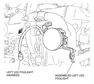
52. Install the assembled left LED foglight as shown.
