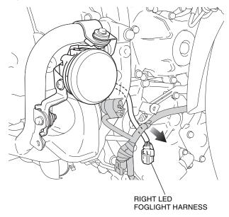
56. Remove the dummy connector as shown.
