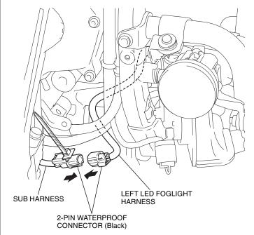
64. Secure the left LED foglight harness with the wire ties as shown.
