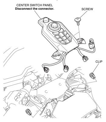
33. Remove the right and left center console panels as shown.
