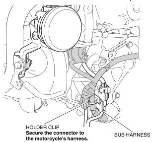
62. Route and secure the sub harness with the wire tie as shown.
