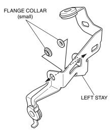
45. Loosely install the assembled left stay to the assembled LED foglight as shown.
