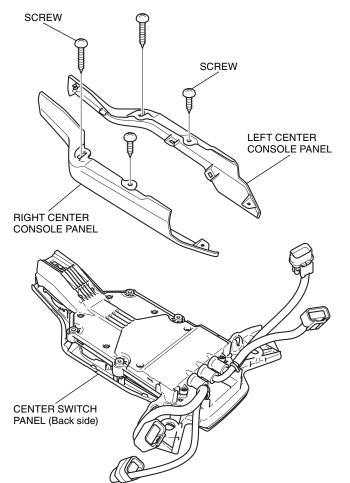
34. Remove the center console garnish as shown.
