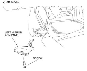
12. Remove the left rear view mirror as shown.
