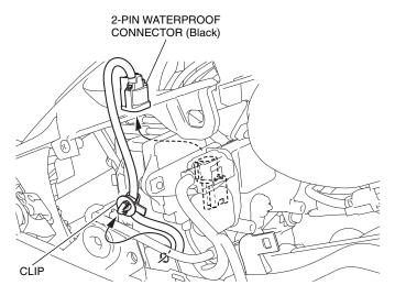
24. Remove the right outer air guide as shown.
