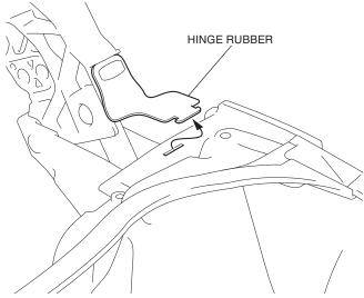
4. Remove the right trunk hinge as shown.
