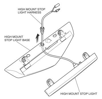
27. Install the high mount stop light as shown.
