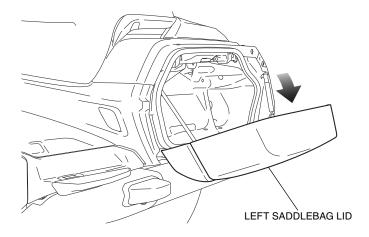
2. Remove the left side cover as shown, and disconnect the negative (-) cable of the battery.
