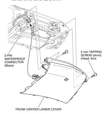
43. Remove the dummy connector as shown. < Right side>
