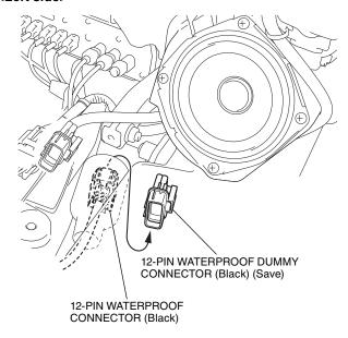
46. Connect the connector as shown.
