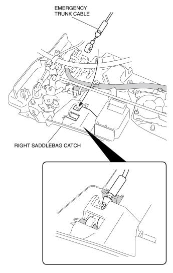
24. Install the radio antenna and right saddlebag catch in the reverse order of removal.
