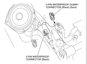
44. Connect the connector as shown.
