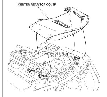
47. Install the clips and 5 mm screws as shown.
