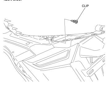
19. Remove the rear fender as shown.
