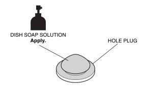
30. Install the hole plug as shown.
