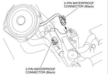
37. Install the dummy connector as shown.
