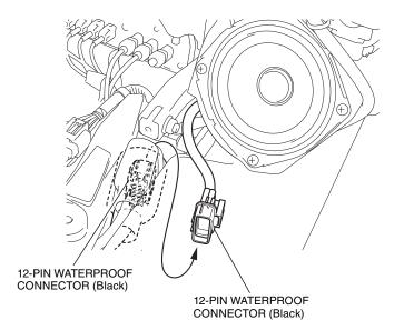
35. Install the dummy connector as shown.
