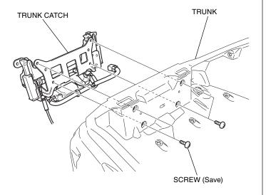
TRUNK CATCH HARNESS 17. Remove the emergency trunk cable from the trunk catch as shown.
