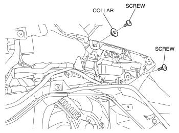
17. Remove the connector as shown.
