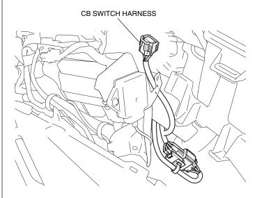
46. Secure the CB switch harness with the wire tie as shown.
