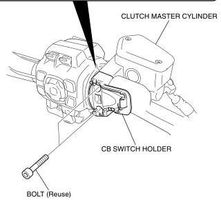
39. Install the CB switch case as shown.
