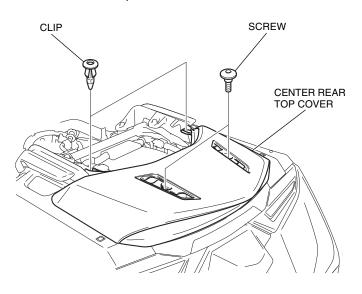
9. Remove the center rear top cover by pulling it firmly up and back as shown.
