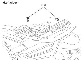
12. Remove the rear fender as shown.
