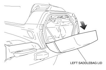
2. Remove the left side cover as shown, and disconnect the battery negative (-) cable.
