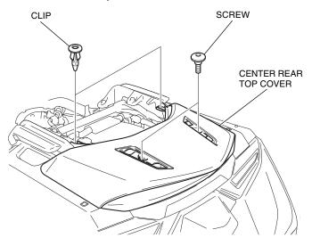
9. Remove the center rear top cover by pulling it firmly back and up as shown.
