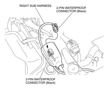
32. Secure the right sub harness with the wire ties as shown.
