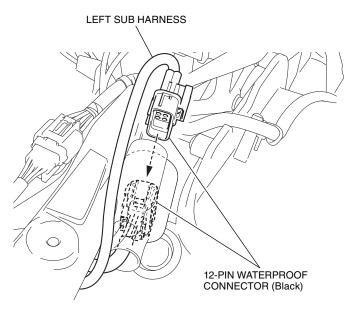
37. Secure the left sub harness with the wire tie as shown.
