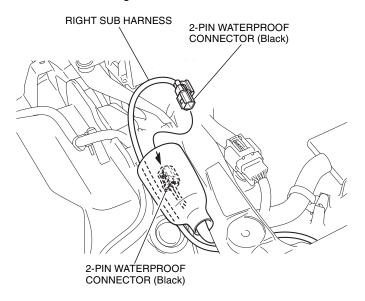
31. Secure the right sub harness with the wire ties as shown.
