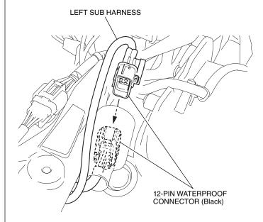
36. Secure the left sub harness with the wire tie as shown.
