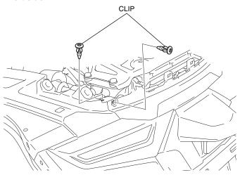
12. Remove the rear fender as shown.
