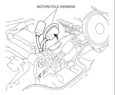
37. Disconnect the connector as shown.
