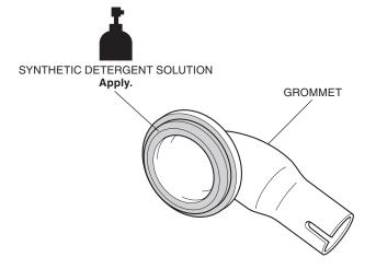
27. Install the grommets as shown.
