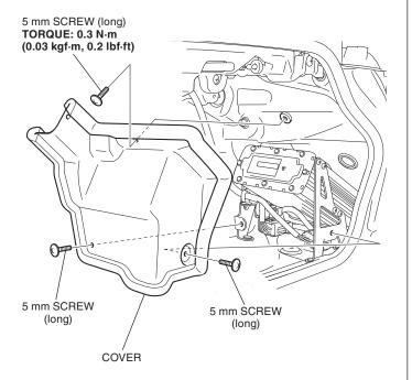
49. Install the 5 mm screw as shown.
