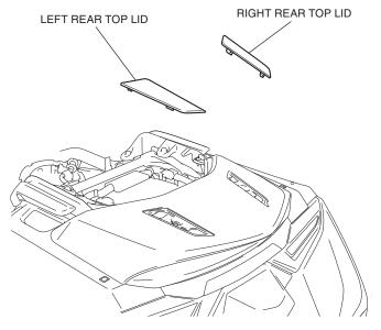
11. Remove the parts as shown.
