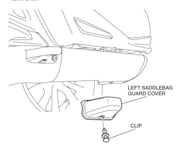
2. Remove the parts as shown.
