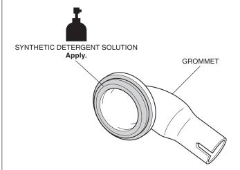
24. Install the grommets as shown.
