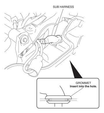
42. Secure the left sub harness with the wire tie as shown.
