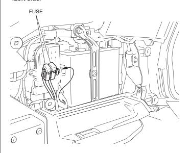
Remove the left passenger step holder cover as shown.
