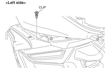
18. Remove the rear fender as shown.
