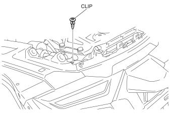
15. Remove the rear fender as shown.
