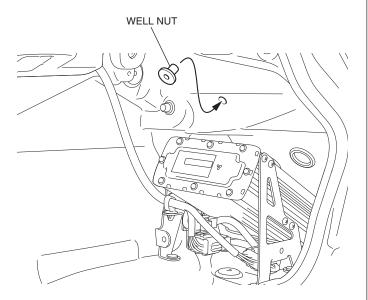
46. Clean the surface of the area shown using isopropyl alcohol.
