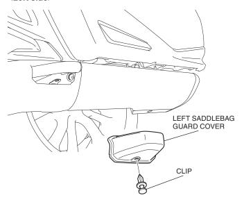
2. Remove the parts as shown.
